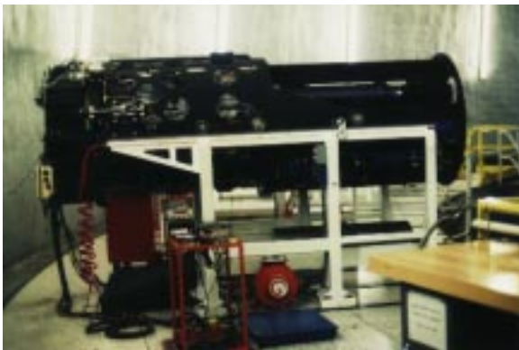
Figure 10: Instruments for the Keck telescope: a. the Near-Infrared Camera (NIRC) in a stowed configuration, and b. the Low Resolution Imaging Spectrograph (LRIS), installed for operation at the Cassegrain focus of the telescope.
