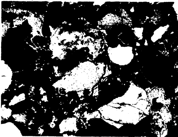
Figure 4.— Back-scattered electron image of sintered lunar simulant basalt (frame width = 500 μm).
