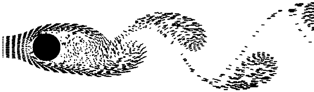
Figure 1. CFD RESULTS FOR KARMAN VORTEX STREET
