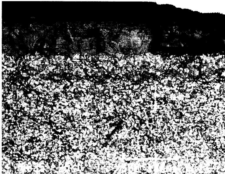
Figure 12. Edge view of amorphous layers on electron emitter surface. This micrograph was taken near the upstream end of the emitter.
