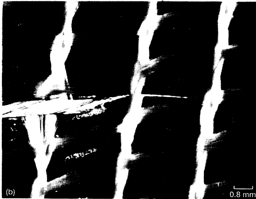
Figure 10. Candidate sample B1.6 after thermal cycling. (a) Close up of purposely cut region showing fine tear which propagated during thermal cycling. (b) Backside of sample showing the tear extending to the second fiber bundle beyond the cut.
