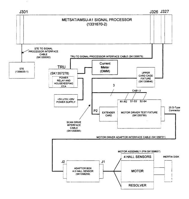
Figure 2 Scan Drive Test Set-Up
