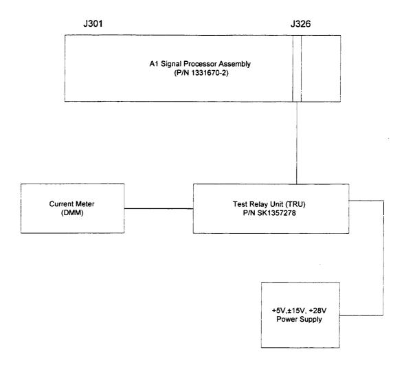
Figure 1. A1 Signal Processor Test Setup
