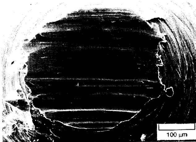
Figure 10.—Wear scar on unlubricated Ti-6Al-4V pin after sliding against high-nickel-content superalloy disk at 2.5 N in vacuum.
