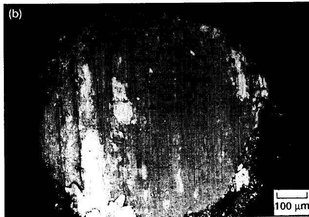
Figure 18.—Wear scar on dry-film-lubricated Ti-6Al-4V pin after sliding against high-nickel-content disk in humid air and then rerun in vacuum.
