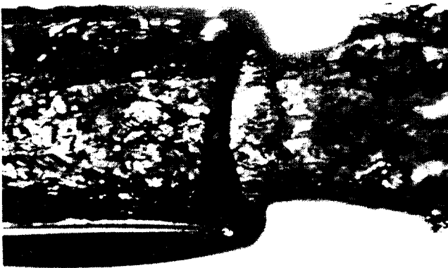
Fig. 2.4.11. Image of Annular flow in tube. Tube length = 9 in.; tube diameter = 0.15 in.; J(\text{H}_2\text{O}) = 3.3 \text{ ft/s} ; J(\text{N}_2) = 234.9 \text{ ft/s} .
