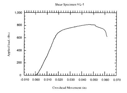
Figure 7. Load vs. crosshead displacement curve for one of the shear test specimens.
