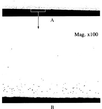
Figure 3. Low (a) and high (b) magnification optical micrographs of beams cross sections revealing inclusion bands. Unetched.
