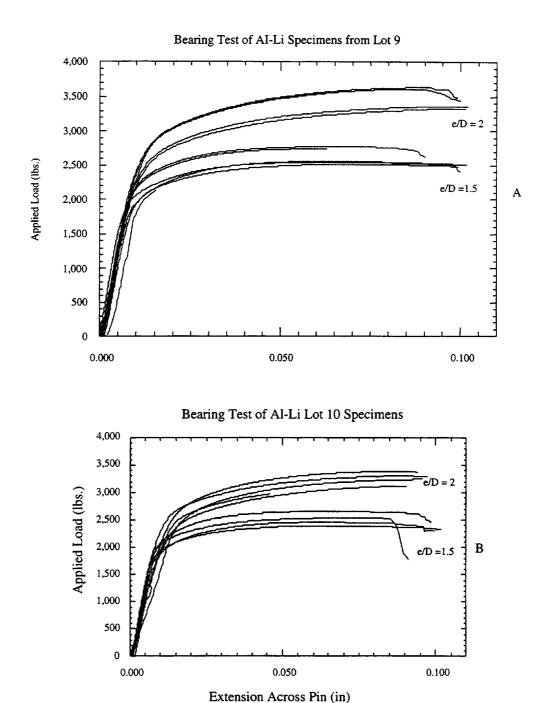
Figure 8. Load vs. displacement curves for the bearing test. There is no noticeable difference in the behavior between Lot 10 (view A) and Lot 9 (view B) specimens.
