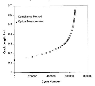
Figure 12. A typical crack length vs. cycle number plot obtained by compliance method and optical measurements.
