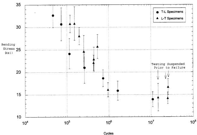
Figure 15. Fatigue life curves for the X2096-TA83 Al-Li alloy extruded beams measured in L and LT orientation.
