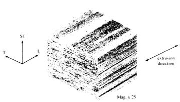
Figure 2. Three dimensional optical micrograph at mid-thickness location in X2096-TA83 extruded beam (20 sec. Graff-Sargent Reagent, Followed by 15 sec. Keller Etch).
