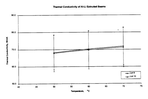
Figure 18. Thermal conductivity as a function of temperature for the Reynolds X2096-T8A3 Al-Li alloy extruded beams.
