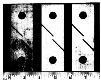
Figure 6. Double slotted single shear test specimens used to measure shear strength of Al-Li extruded beams. A complete description of these tests can be found in Ref. 2.
