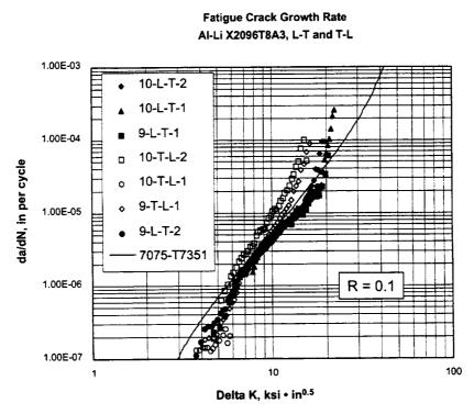
Figure 13. Shows a plot of da/dN vs. ΔK for the test specimens machined from the extruded beams of X2096-T8A3 Al-Li alloy. Specimens ID indicates the lot, orientation, and the specimen number.
