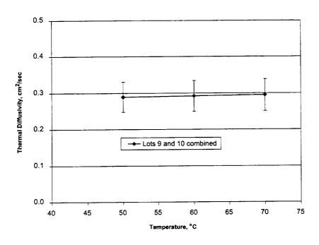
Figure 17. Thermal diffusivity as a function of temperature for the Reynolds X2096-T8A3 Al-Li alloy extruded beams.
