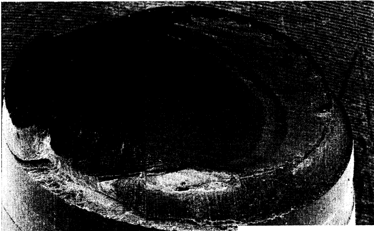
Figure 18. Secondary electron image of fracture surface from a typical LCF specimen.
