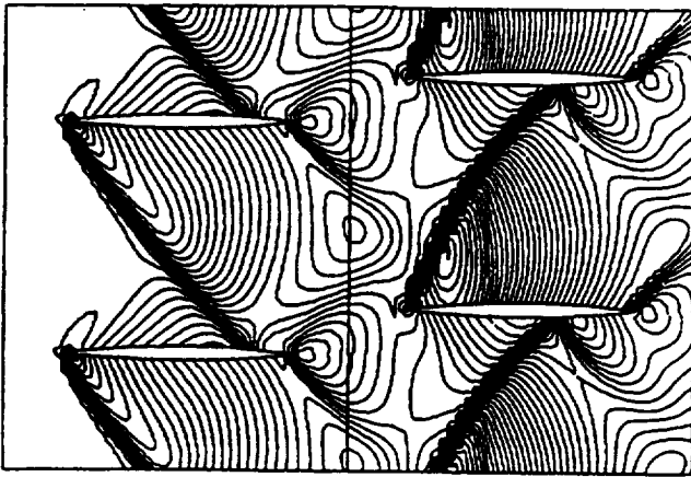
Figure 7.31 : Pressure Contours for Case (a) and the end of 4.2 cycles from [52]
