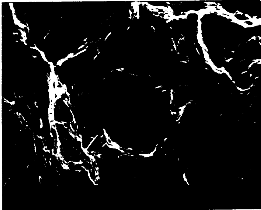
Figure 3.12. Fracture surface of specimen S-11 at 300x (top) and 2000x (bottom) showing tear ridges and ductile dimples at precipitate particles
