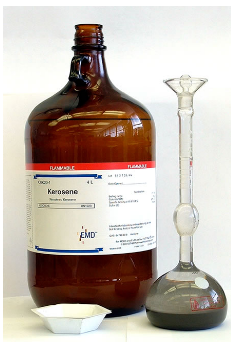
Figure 4.5. Test Set-Up for the Cement Density Determination.
