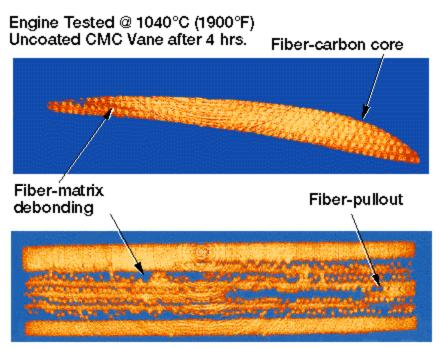
Tensile Tested @ 21°C (70°F) 5-Ply CMC After Failure 12.7mm (0.5 inch) wide
