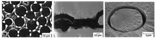
Oxidation behavior of model composites with BN layers. Top: At 816 °C for 100 hr with low water vapor, BN deposited at a low temperature forms borosilicate. Middle: At 900 °C for 140 hr with low water vapor, BN deposited at a high temperature remains intact. Bottom: At 500 °C for 100 hr with water vapor, BN deposited at a low temperature is volatilized.
