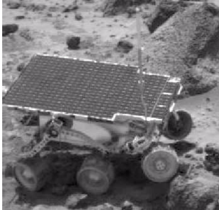
Sojourner rover on sol 41. Dust is uniform on the wheel drive surface. (Wheel detail is obscured.)
