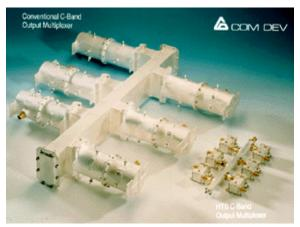
Comparison of a conventional C-band output multiplexer with the HTS/dielectric multiplexer developed by ComDev and DuPont under a cooperative agreement with NASA Lewis and the Defense Advanced Research Projects Agency (DARPA). Both multiplexers can handle 24 W of microwave power per channel.
