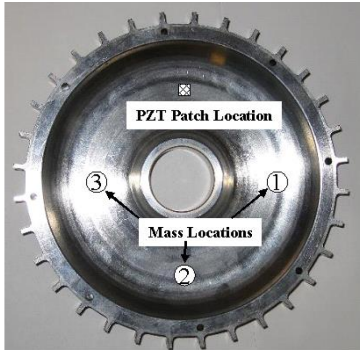
Figure 4. Disk specimen with mass and PZT sensor locations.
