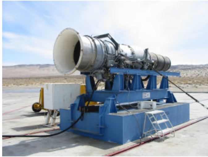
Figure 1. TF-41 engine and test stand at China Lake, CA.
