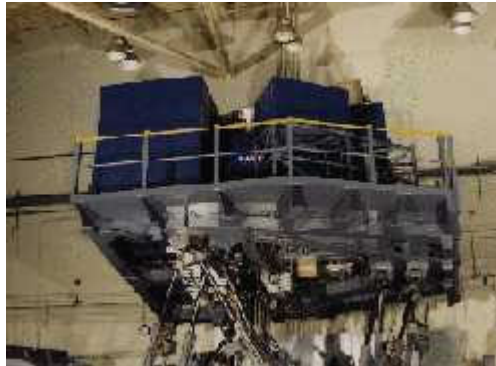
Figure 2.1. NASA Langley Visual Motion Simulator (VMS). NASA Langley Research Center, Hampton, Virginia.
