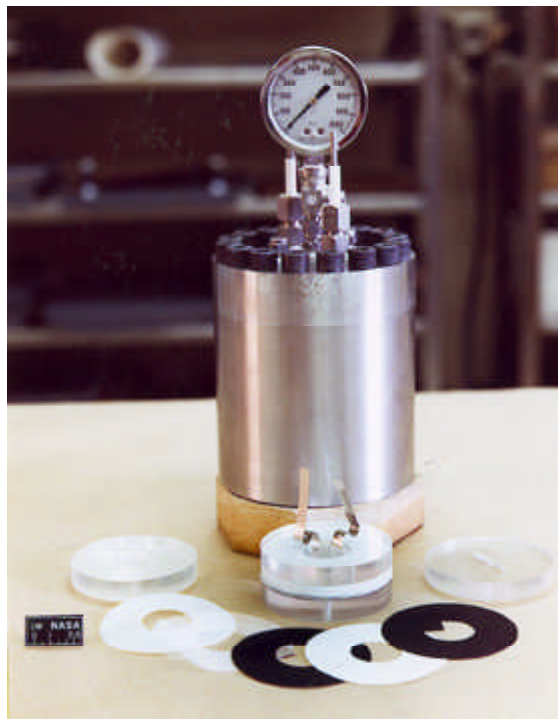
Nickel-hydrogen boilerplate cell.
