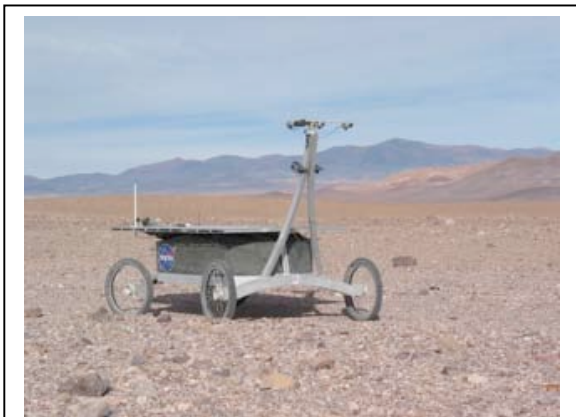
Fig. 4. Zoë robot in the Atacama conducting long-distance traverse with full instrument payload to characterize geology and biology of site (2004).
