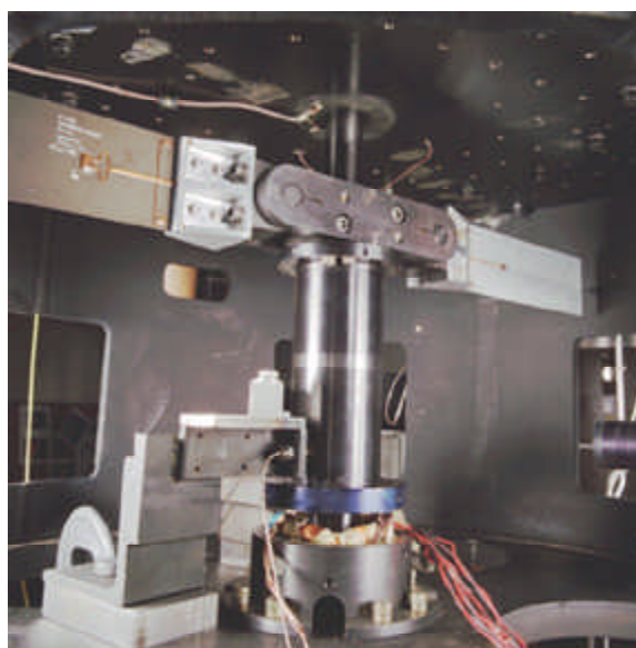
Radial magnetic bearing in NASA Lewis' Dynamic Spin Rig showing viscoelastic damped
