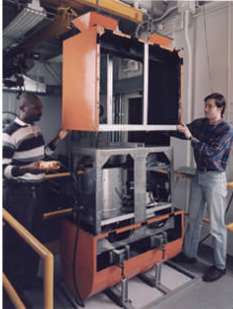
The top of the drag shield is lowered into position over a combustion experiment from the University of Michigan prior to a test in Lewis' 2.2-Second Drop Tower.
