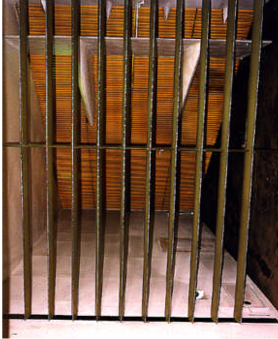
New spray bar system for Lewis' Icing Research Tunnel as seen from the test section.
