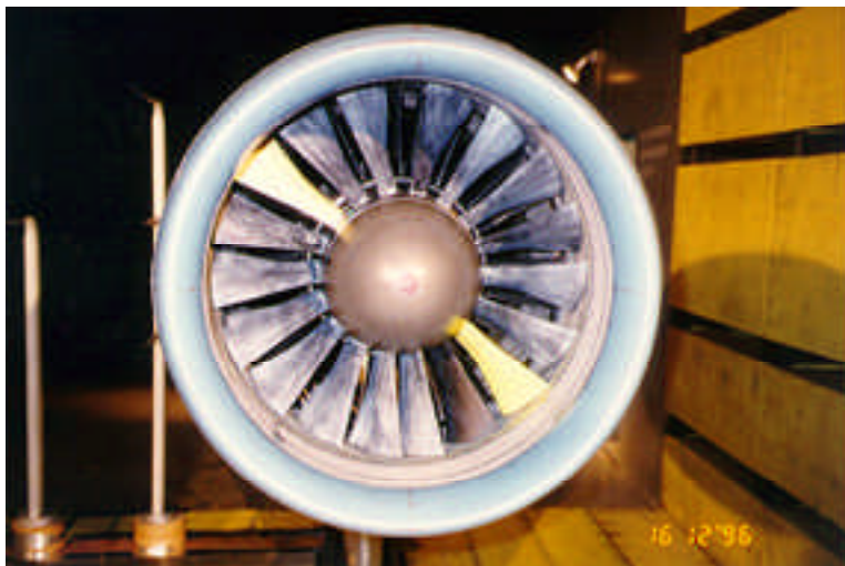
Fan rig mounted in Lewis' 9- by 15-Foot Low-Speed Wind Tunnel. Blades are painted with TSP and PSP.
