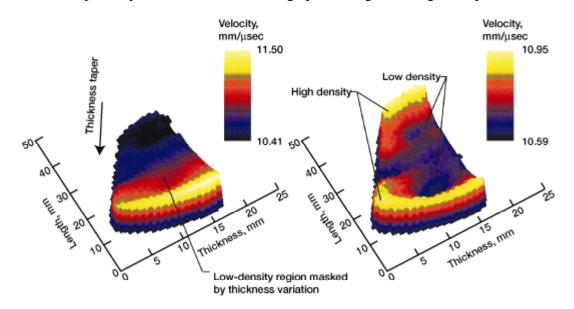
Conventional ultrasonic imaging versus thickness-independent ultrasonic imaging for silicon nitride monolithic ceramic with pore fraction variations and 10-percent thickness variation. Left: Conventional ultrasonic image. Thickness effect not eliminated; defects not revealed. Right: New thickness-independent ultrasonic imaging. Thickness eliminated; defects revealed.
