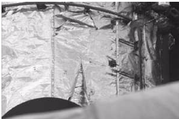
Hubble Space Telescope light shield sample retrieved during the second servicing mission; shown prior to removal.
