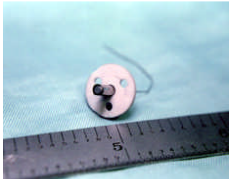
Support sleeve and ceramic disk mounting for 0.065-in. cathode scale.
