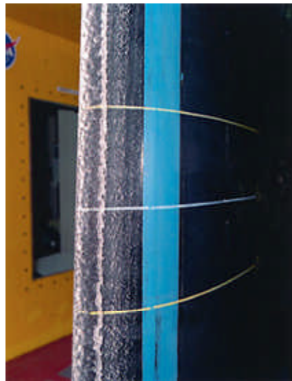
Ice accreted during the testing of the EMB-120 wing in Lewis' Icing Research Tunnel.
