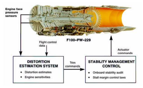
Distortion tolerant control. (Engine cutaway copyright Pratt & Whitney; used with permission.)
