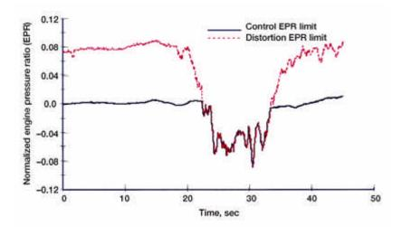
*In-flight fan distortion accommodation.*
