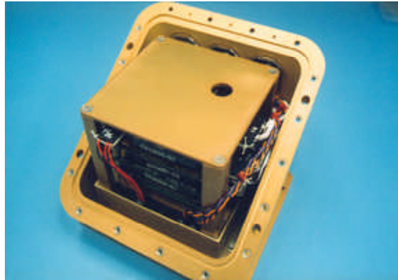
SAMS-FF-4: SAMS-FF control and data acquisition unit in hermetic enclosure.
