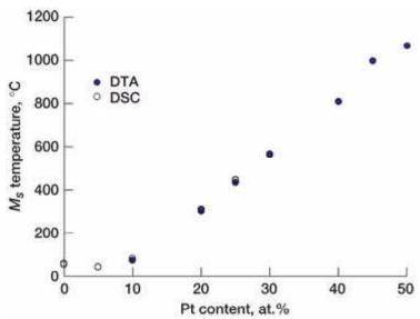
Martensitic start temperature,  $M_s$ , for  $Ti_{50}Ni_{50-x}Pt_x$  alloys as a function of Pt content. The initial region of focus for high-temperature actuators for aerospace applications includes alloys containing 15 to 35 at.% Pt for DTA, differential thermal analysis, and DSC, differential scanning calorimetry.
