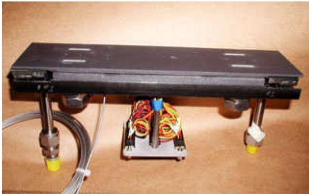
Subscale 2.5- by 10-in. maintainable panel assembly before testing in Glenn's Research Combustion Lab.
