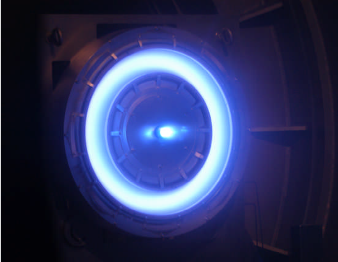
NASA-457M Hall thruster operating at 65 kW on krypton propellant. Electric propulsion device with a 457-mm outside-diameter annular discharge chamber.
