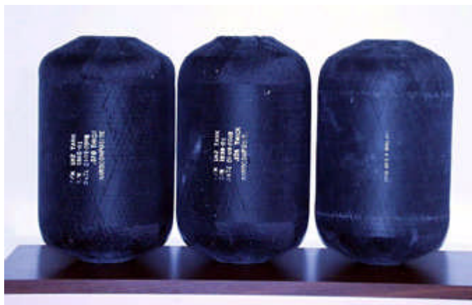
Polymer/silicate nanocomposite tanks tested for helium permeability. Long description.
