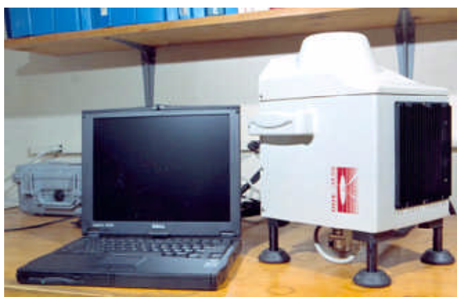
Portable infrared reflectometer for evaluating emittance.
