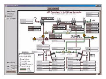
The schematic portion of the viewing system provides users with access to values for key test parameters during a user-specified time interval. Sensor failure information also is given.
