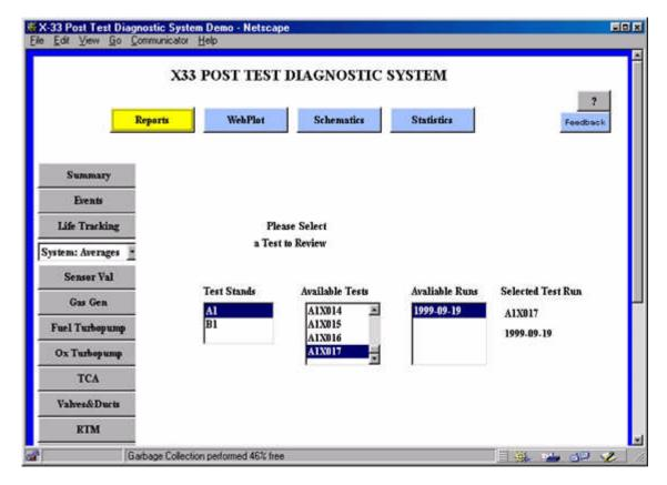
The Web-based viewing system allows users to access PTDS analysis results and data through reports, an interactive plotting tool called WebPlot, schematics, and an interactive statistics tool.
