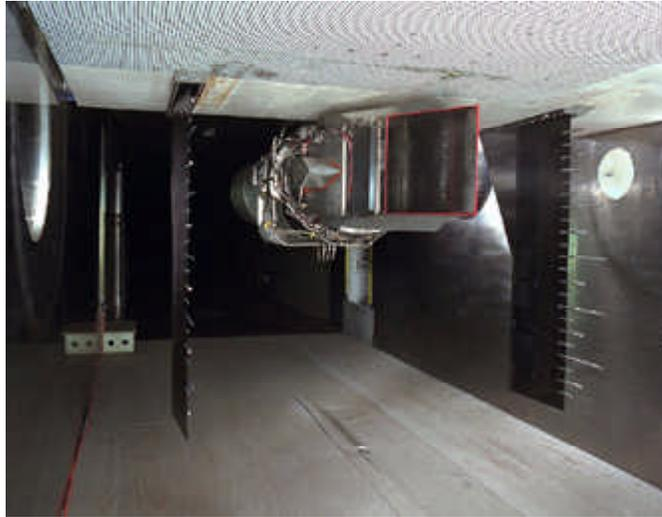
*View of test model and instrumentation installed in Glenn's 10- by 10- Foot Supersonic Wind Tunnel.*
