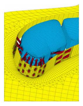
Cut-through view of the DRAGON grid in the leading-edge region of a film-cooled turbine vane, showing the internal plenums and coolant holes inside the vane.
