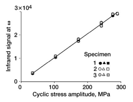
First harmonic (W) infrared signal output at various stress amplitudes ( $S_m = 0$ ) for TIMETAL21S. Indicated is the linear relationship of the TSA signal to the cyclic stress amplitude for a fixed mean stress. Mean stress variations would affect the data by changing the slope of the line.
