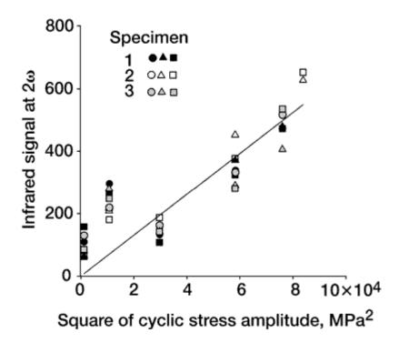
Second harmonic (2w) infrared signal output at various stress amplitudes ( $S_m = 0$ ). Indicated is the linear relationship of the TSA signal to the square of the cyclic stress amplitude. The second harmonic TSA response is independent of the cyclic mean stresses.
