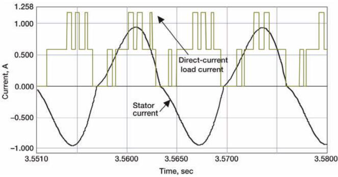
Typical output waveform of the simulation model. This shows the ac flowing through the stator windings of TDC 14 and the direct current (dc) dissipated in the ZDC.
