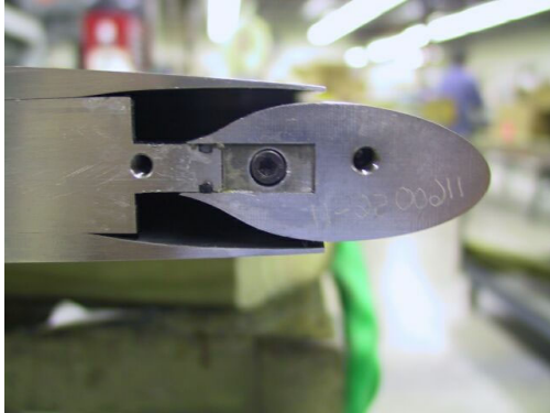
Figure 4 - End View of a Coanda Surface and Aft Surfaces
