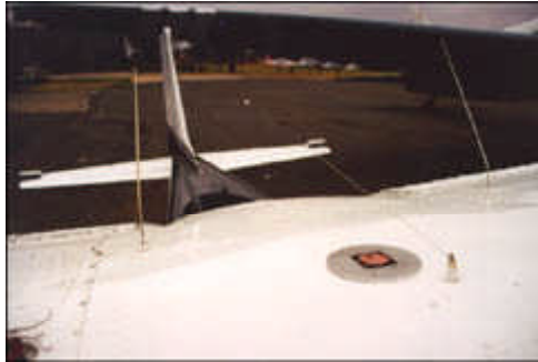
Rockwell Collins patch antenna mounted on the fuselage of a Cessna-172 aircraft.
