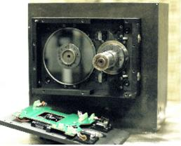
Optical and electronic components of the new transmission error measurement system. Note the reflections in the two mirrorlike gratings. The sizes of the gratings are proportional to the size of the gears, which have a 1.8:1 ratio.
