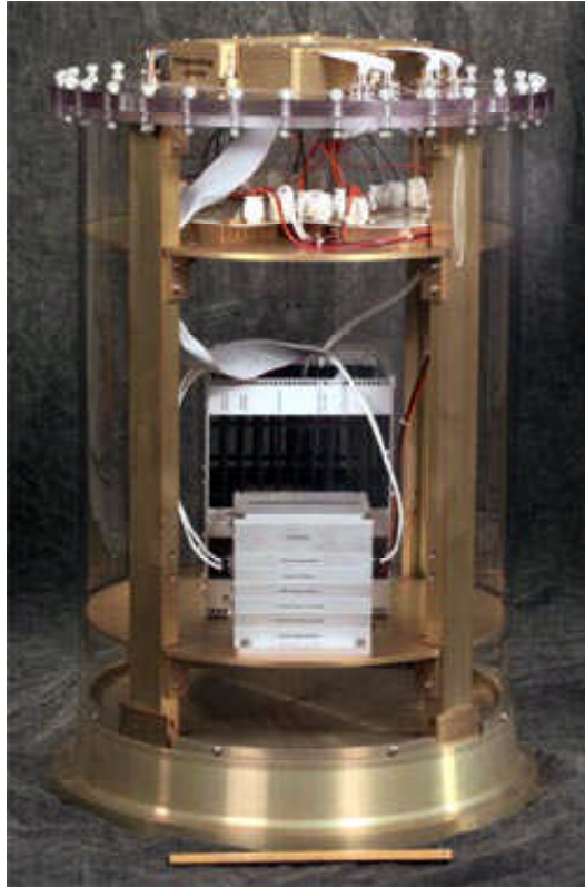
Flight mockup of the Direct Data Distribution (D 3 ) experiment in a GSFC Hitchhiker-G Canister.
