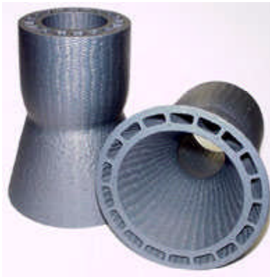
Silicon-carbide-fiber-reinforced silicon carbide matrix composites with woven cooling tubes.
