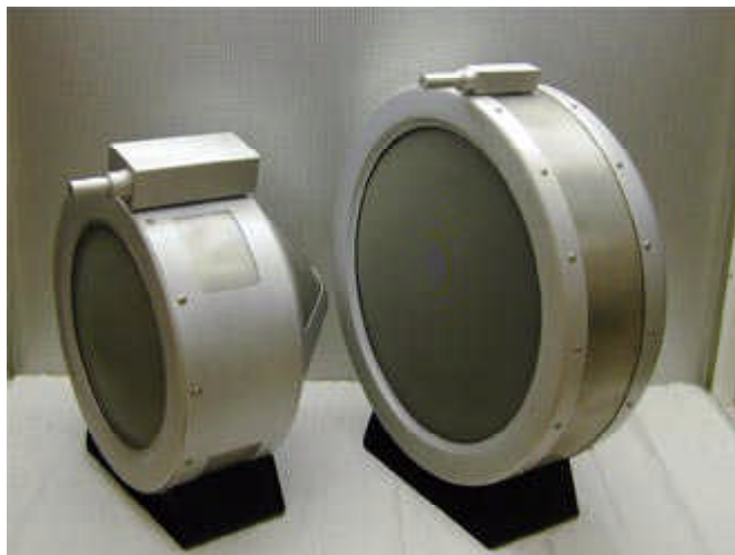
Left: Deep Space 1 thruster. Right: 40-cm engine.
