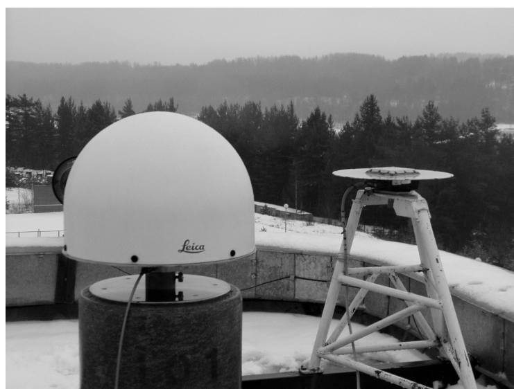
Figure 2. GPS receiver Trimble 4000SST was replaced with Leica SR520 with choke ring antenna LEIAT 504 on Dec 1, 2004.
