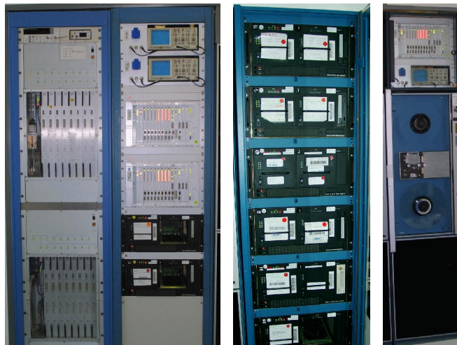
Figure 1. Left: correlator surrounded by two Mark 5 playback units and two station units. Center: six rack-mounted Mark 5 playback units. Right: tape drive with station unit on top.
