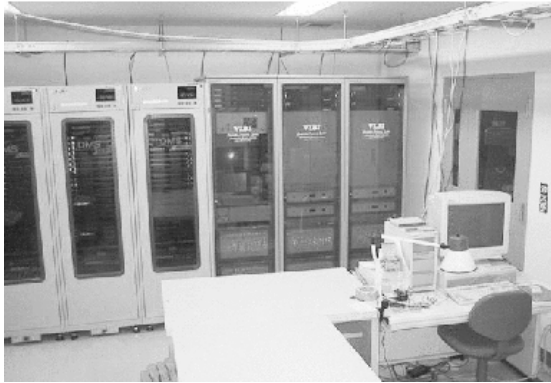
Figure 1. KSP Correlator room. The KSP hardware-correlation system, which is capable of processing 4 stations and 6 baselines of tape-based VLBI data, is sometimes operated for domestic geodetic VLBI data processing.
