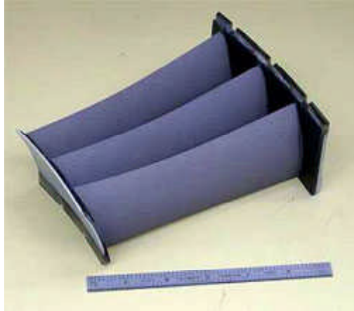
NASA Glenn erosion coating on a PMC inlet guide vane section.
