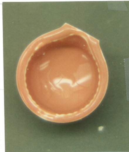
9. Photograph of color enhanced phenyl methyl silicone vacuum degassed after mixing in air and dispensed in vacuum/zero-net gravity facility.
