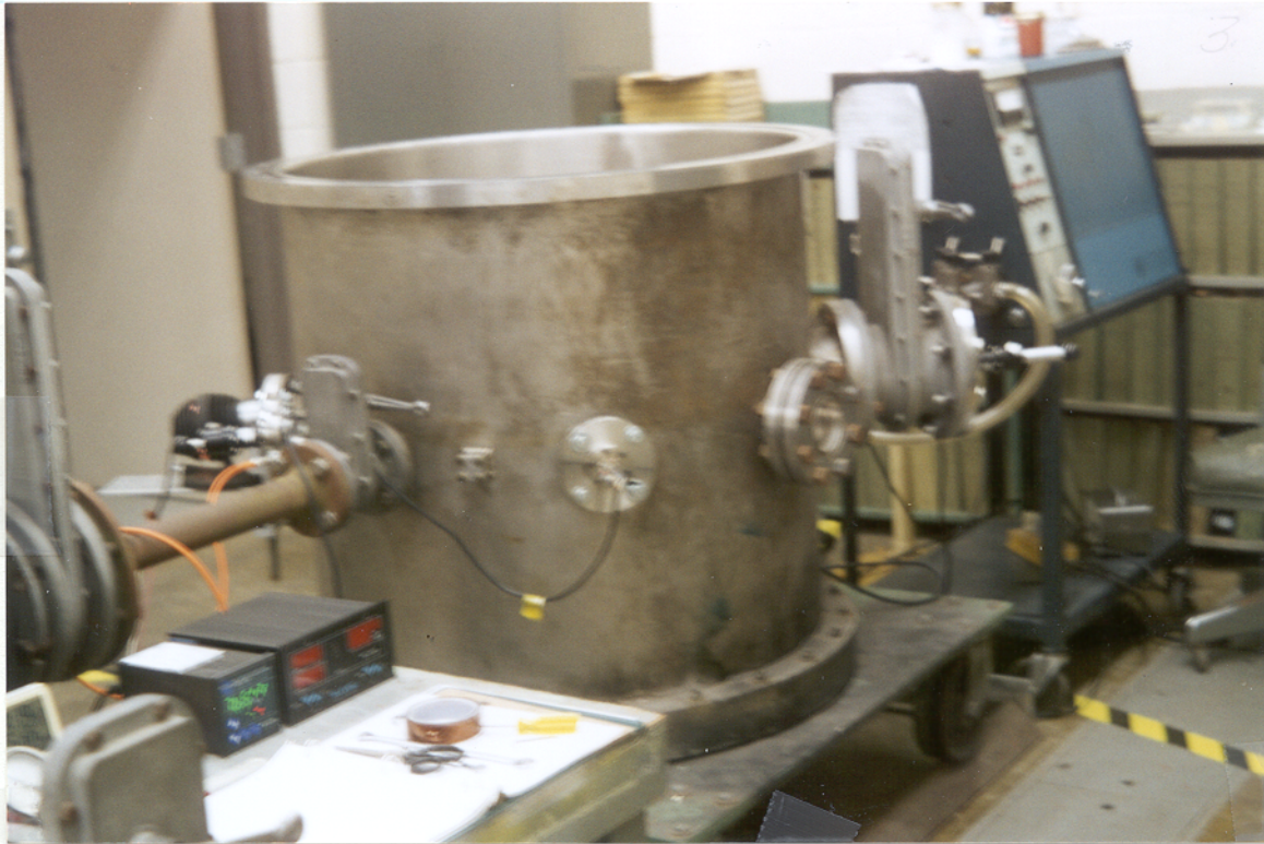
4. 1 m x 1m top loading vacuum chamber (top off).
